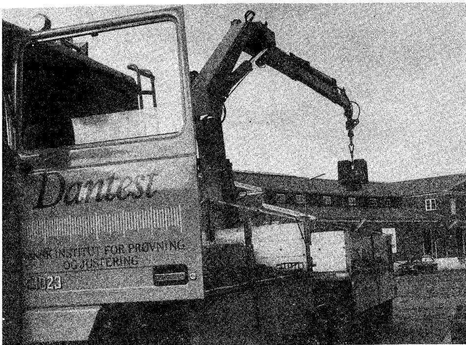
Fig. 2 — The special design of the weights is an important condition for quick operations with the hydraulic crane.
