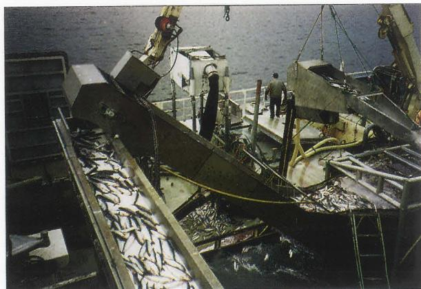
Fig. 4 Arrangement for pumping the fish from the vessel into the dockside bin. Conveyors bring the fish into the plant.
