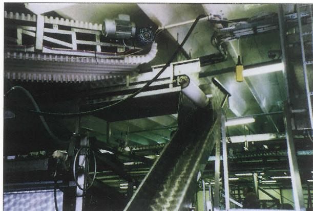
Fig. 3 Scanvaegt belt weigher, the driving drum. The reversible conveyor and the chute which are used to carry out the in-situ material test.
