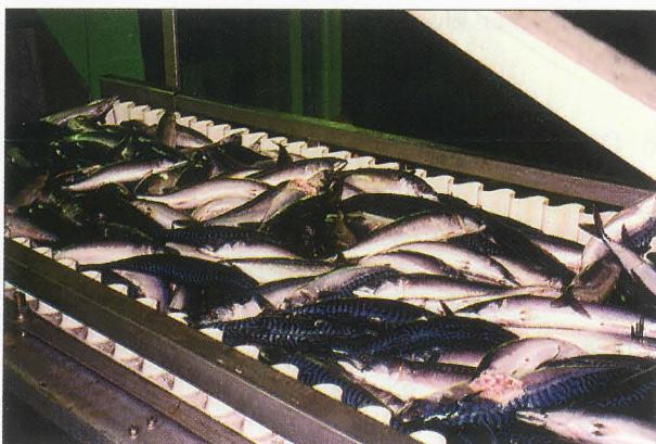
Fig. 7 Mackerel spread symmetrically on the weighing belt
