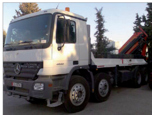
Figure 7 Vehicle and telescopic crane provided with 20 T of dead weight for the verification of weighbridges
