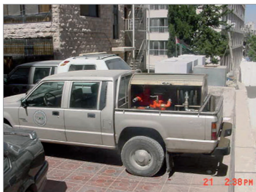
Figure 8 Mobile master flow meter used for unannounced verification of road fuel tankers
