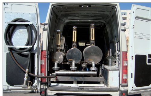
Figure 10 Mobile working volume standards 1, 2, 5, 10, 20, 50, 100, 200 L for verifying fuel dispensers
