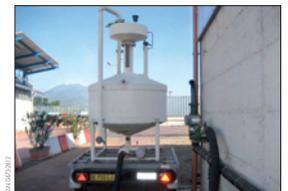
Master meter used for the verification of bottom loading road tankers in Naples
