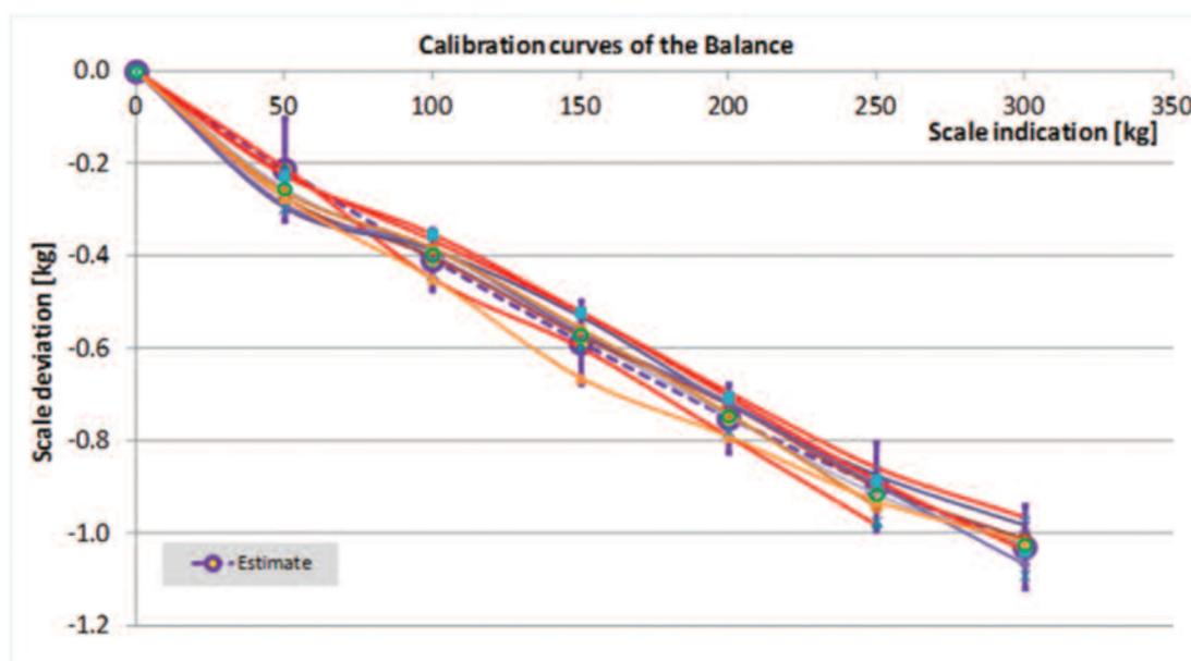
Figure 4 Balance calibration curves and uncertainty bars
