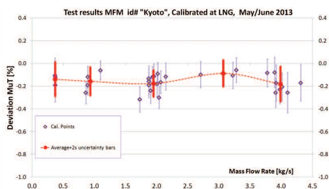
Figure 11 Results of LNG calibration of flow meter D
