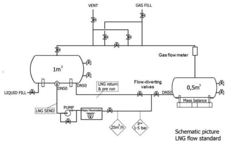
Figure 2 Schematic picture of the primary LNG flow standard
