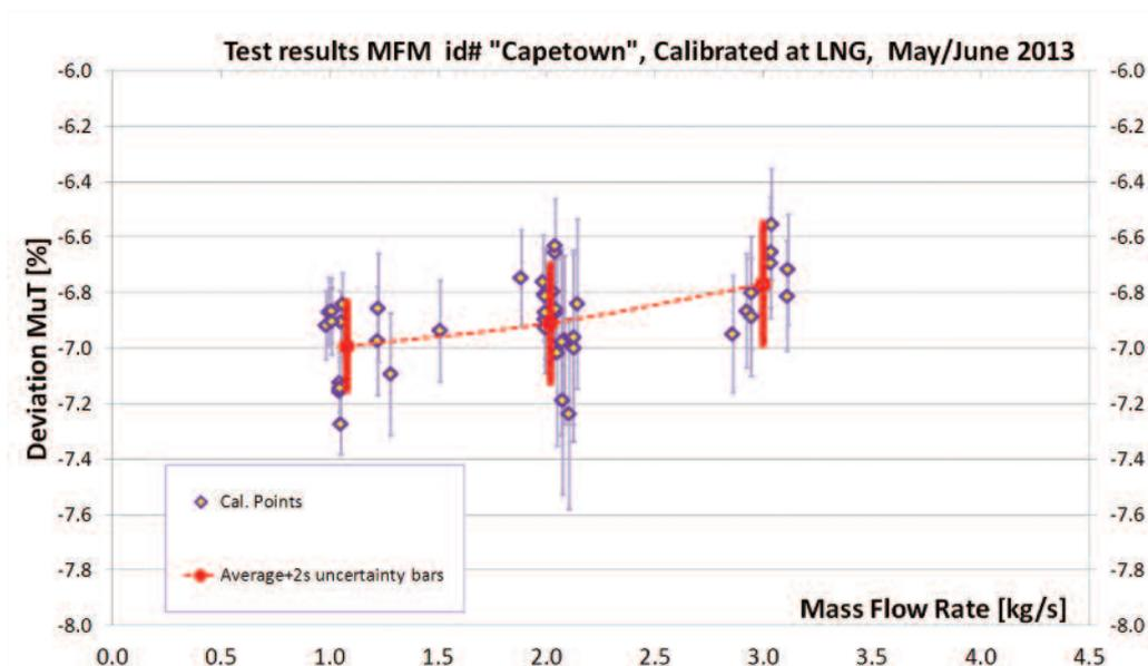
Figure 7 Results of LNG calibration of meter A
