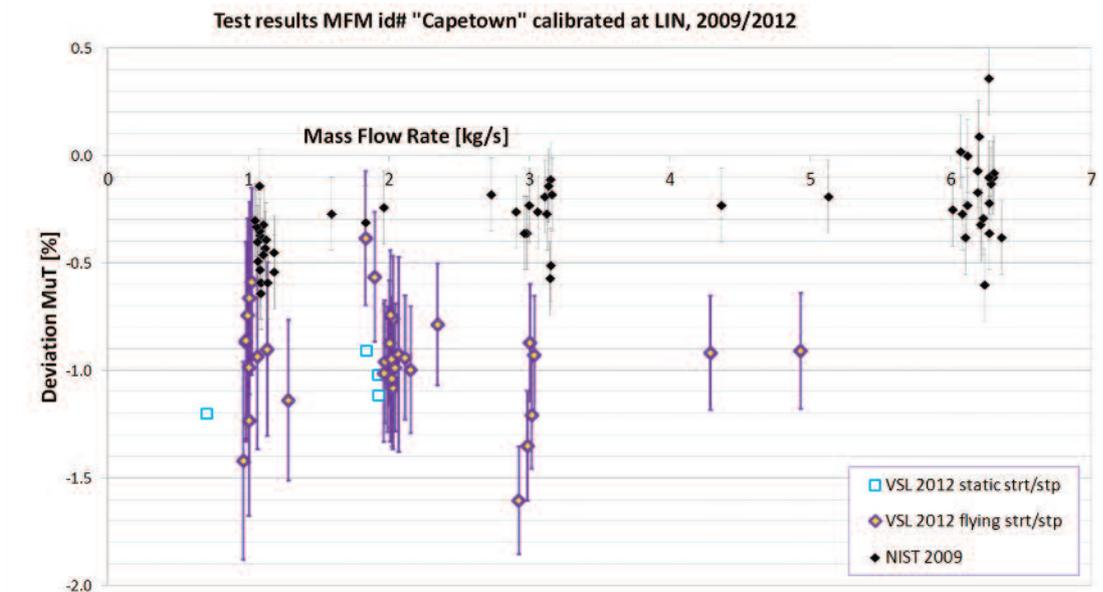
Figure 6 Results of LIN calibrations at different facilities
