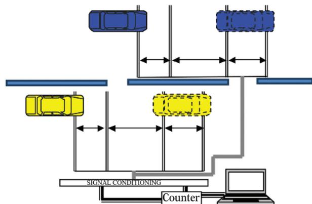
Fig. 3 Arrangement of the sensors for the measurement of the different speeds
