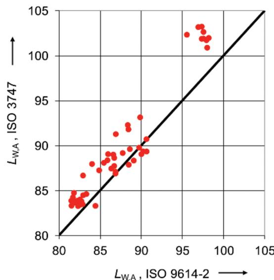
Figure 2: A-weighted sound power levels of five different machines measured each by 8 different teams with two different methods (ISO 3747 and ISO 9614-2), measurement results from [16], analysis from [17].
