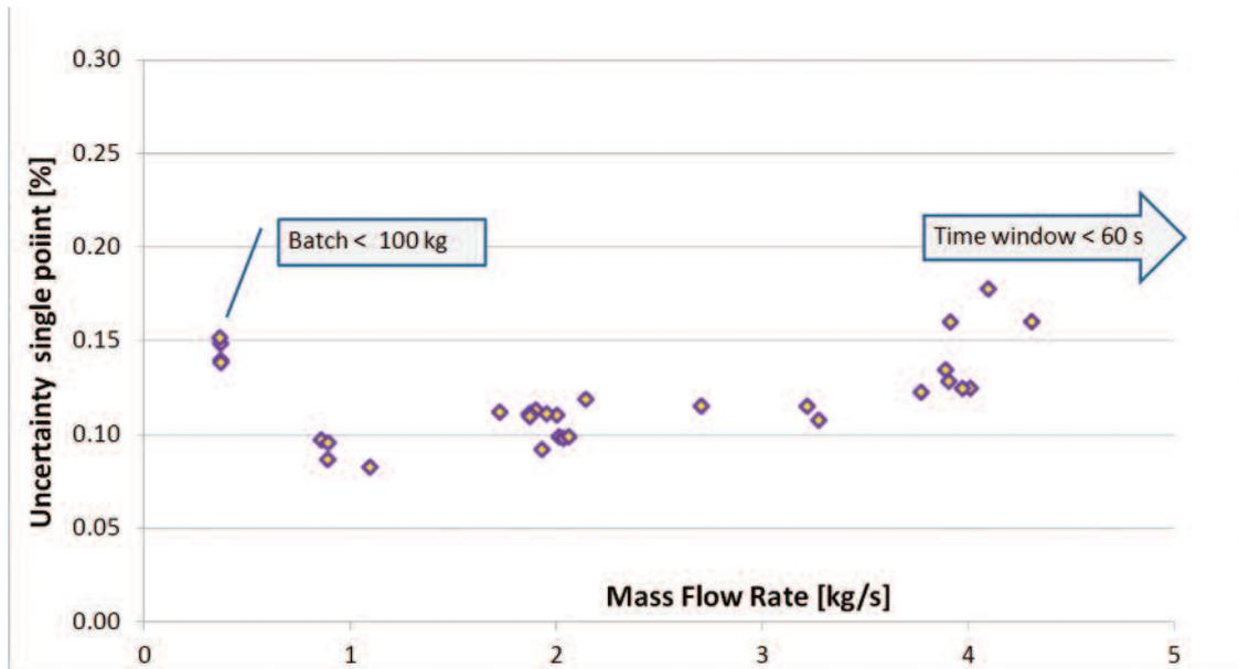
Figure 5 Typical uncertainties of reference mass flow rate
