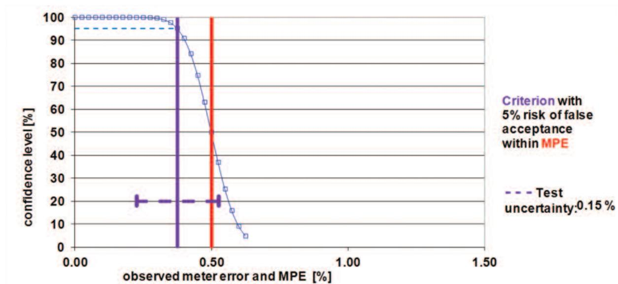
Figure 10 Pass criterion of meter under test at 5 % risk of false acceptance, MPE = 0.5 %, uncertainty = 0.15 %
