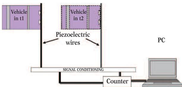
Fig. 2b The system records the signals and measures the time between them
