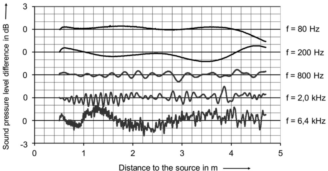
Figure 1: Difference between measured sound pressure levels and the ideal free field in a high quality hemianechoic room as a function of the distance to a point source. The standing wave pattern is clearly visible.
