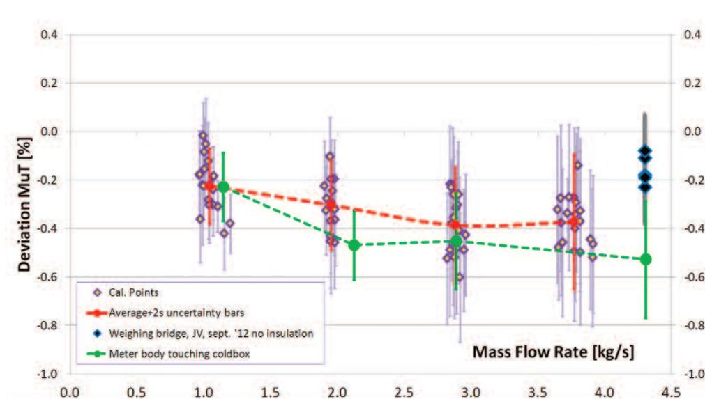
Figure 9 Results of LNG calibration of meter C
