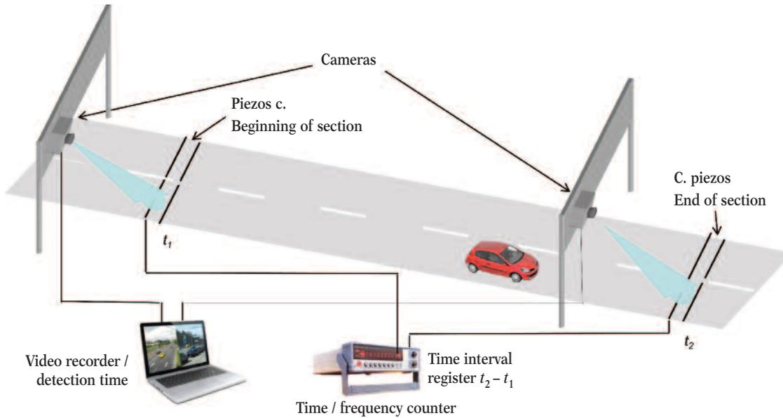
Fig. 2a Arrangement of the sensors for average speeds
