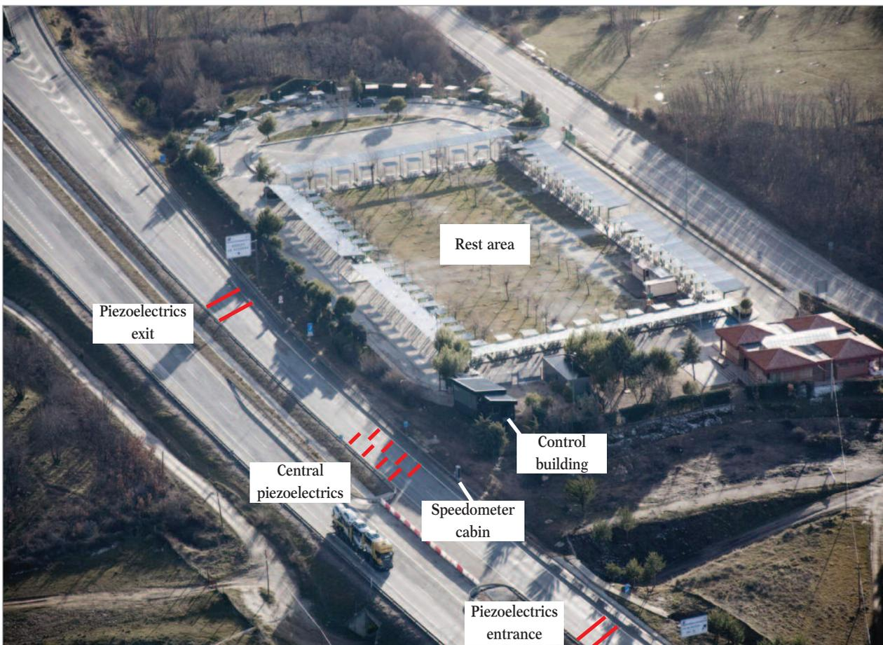
Fig. 10 CEM's facilities in Horcajo de la Sierra (Madrid), for speed measurements
