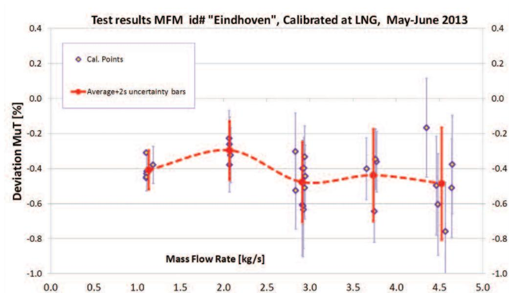
Figure 8 Results of LNG calibration of meter B
