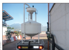
Master meter used for the verification of bottom loading road tankers in Naples
