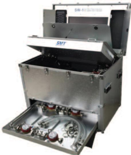
Figure 3 Portable test equipment for a heat meter
