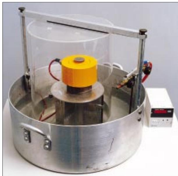
The barometric pressure chamber (see 2.6)
