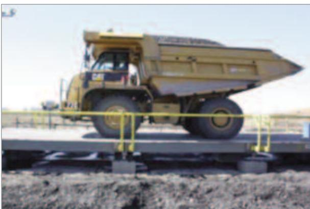
Figure 2 A pitless mounting scale placed above ground [3]
