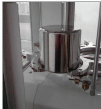
Fig. 1 Reference standard of 1 kg, Ni81
