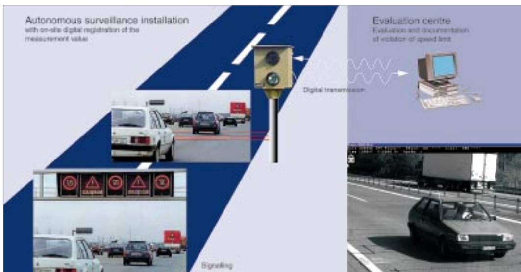
Figure 3 Scheme showing the principle of a traffic surveillance system with a variable speed limit controlled by a traffic regulation system. The measurement values are transmitted to a center for evaluation, where they are stored (Illustration: METAS)
