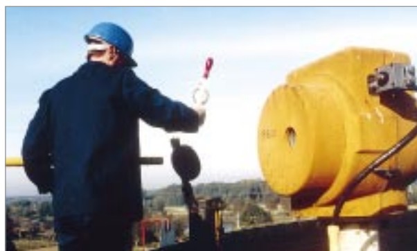
Fig. 6 Manual measurement of the liquid level using graduated tape
