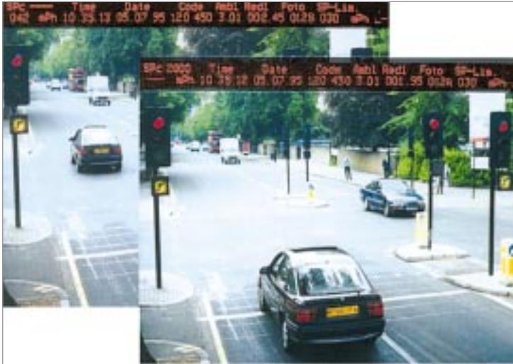
Figure 2 Red light and speed surveillance with on site double image on wet film (Photo: METAS)
