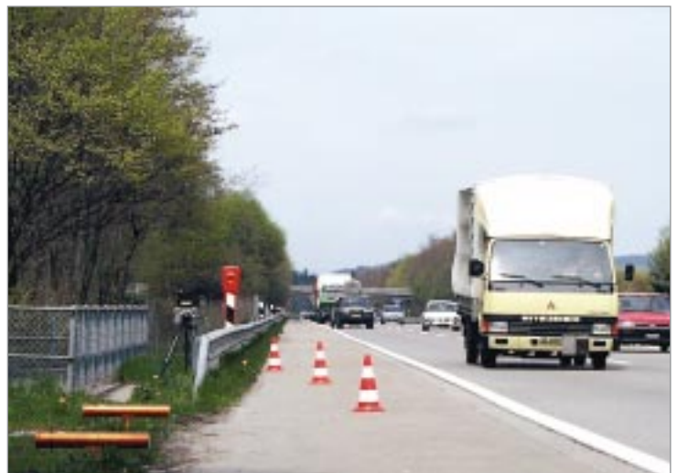
Fig. 1 Speed measuring instruments are compared with the METAS reference installation under realistic traffic conditions (Photo: METAS)
