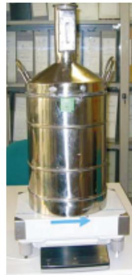
Setup for the indirect calibration of standard volume measures
